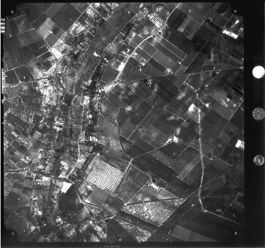
Fig. 3.12 Aerial photograph, original dimension 23 cm × 23 cm with evidence of the flight parameters, the fiducial marks in the corners and the photograph number
