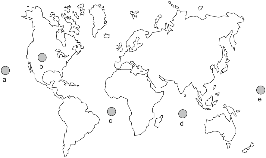
Fig. 7.2 World geographical dislocation of the control stations: (a) Hawaii; (b) Colorado Springs; (c) Ascension; (d) Diego Garcia; (e) Kwaialein
