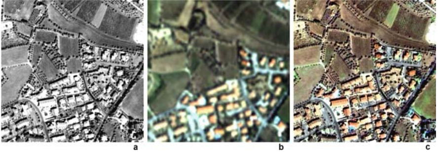
Plate 8.6 The fusion of two images by means of the pan-sharpening technique; a panchromatic image (better geometric resolution) is combined with the 3 multispectral bands (better spectral resolution) of the same scene obtaining a new synthetic image with enhanced geometric and spectral resolutions
