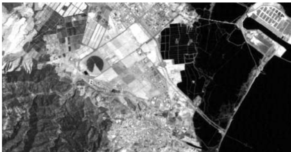
Fig. 8.37 The size of different objects in a scene contributes to their interpretation. In the centre: circular agricultural field with rotating wing irrigation system
