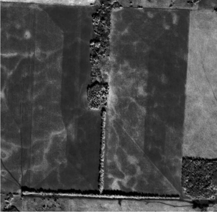
Fig. 8.43 The changing height of the horizontal line of trees is measurable from the shadow projection on the soil
