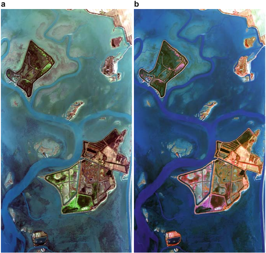
Plate 6.2 Two images of the same area in true colour, a , and false colour, b . In b the vegetation is represented by hue of red and magenta . The water, with very low reflection in the red and infrared , has blue-black colour. Grado Lagoon, Italy
