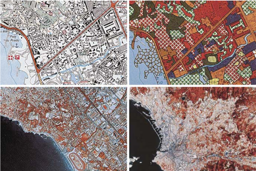
Plate 10.1 Example of ancillary data used for the realization of the CORINE program; (a) topographic map 1:25,000, (b) Land use/land cover map, (c) aerial photograph 1:50,000, (d) satellite image colour composite with overlay of the land use map
